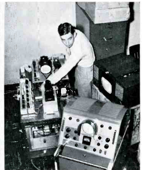
(Left): Ass't Station Engineer Robert Barnes checks the FM transmitter. Its 3 kw output becomes an effective 15 kw through the use of a high-gain super-turnstile triplex antenna. (Right): Transmitter Engineer John Rogers adjusts the flying spot scanner, used to "pick up" test patterns, slides, and may be used to superimpose a still picture on any other television picture, still or moving. The cathode ray tube above Rogers' hand is the source of the flying spot. The scanning light beam from the C-R tube focus through a slide-type picture mounted in the slide viewer in front of the tube; passing through the slide, the light focuses on a photo-electric cell, whose output constitutes the video signal representing the slide picture.
