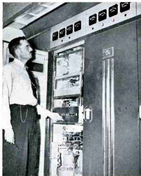
(Left): Ass't Station Engineer Robert Barnes checks the FM transmitter. Its 3 kw output becomes an effective 15 kw through the use of a high-gain super-turnstile triplex antenna. (Right): Transmitter Engineer John Rogers adjusts the flying spot scanner, used to "pick up" test patterns, slides, and may be used to superimpose a still picture on any other television picture, still or moving. The cathode ray tube above Rogers' hand is the source of the flying spot. The scanning light beam from the C-R tube focus through a slide-type picture mounted in the slide viewer in front of the tube; passing through the slide, the light focuses on a photo-electric cell, whose output constitutes the video signal representing the slide picture.
